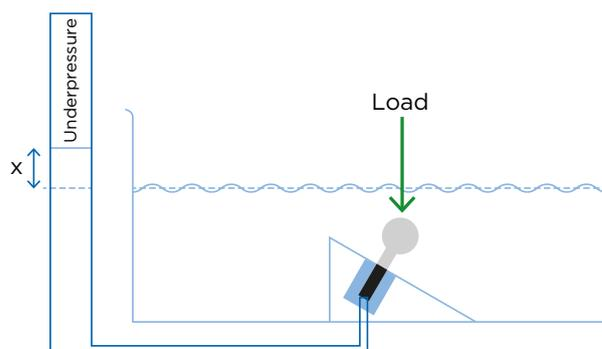
A schematic illustration of the Dentsply Sirona Implants leak test method. The implant and abutment are mounted according to the 30° off-axis method. The underpressure is created through a drilled hole at the bottom of the implant. Fluid leakage can be detected through a rise of the fluid column, which is schematically illustrated as “x”.
