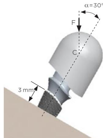
Test setup per ISO 14801:2007. The OsseoSpeed Profile EV implant - abutment assemblies were tested at a 30° angle with the implant embedded to a level 3 mm below the implant shoulder (i.e., nominal bone level). A hemispherical test cap (C) was placed on top of the abutment to ensure proper load (F) distribution.
