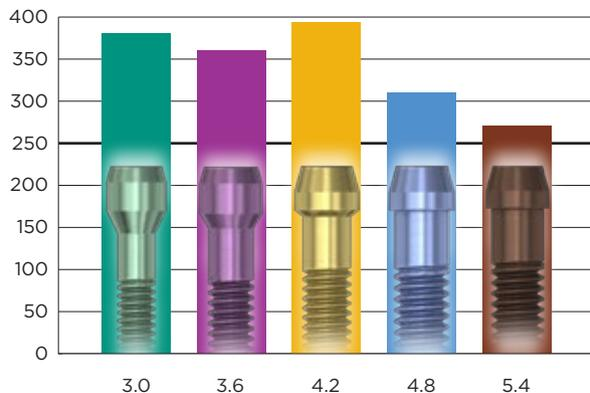
All abutment screws for Astra Tech Implant System EV exceeded the preload of at least 250 N at the tightening torque of 25 Ncm.
