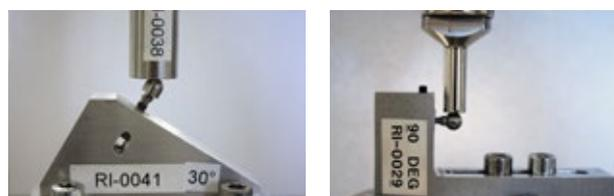
30° off-axis load method (ISO 14801:2007) and Dentsply Sirona 90° off-axis load method.
